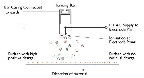
of the material the electrons will be exchanged and the surface will be neutralised.
